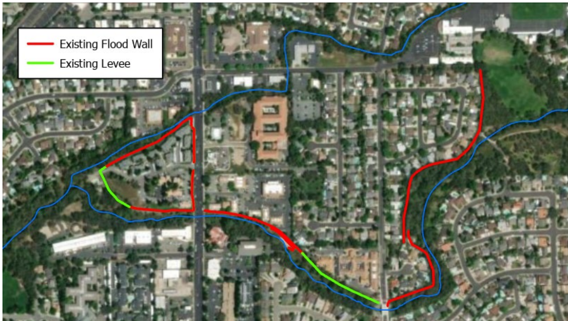
Figure 10. Existing Flood Control Structures in the Study Area.
